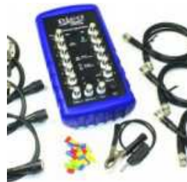
Mixmaster 12-Channel Automotive Signal Mixer
